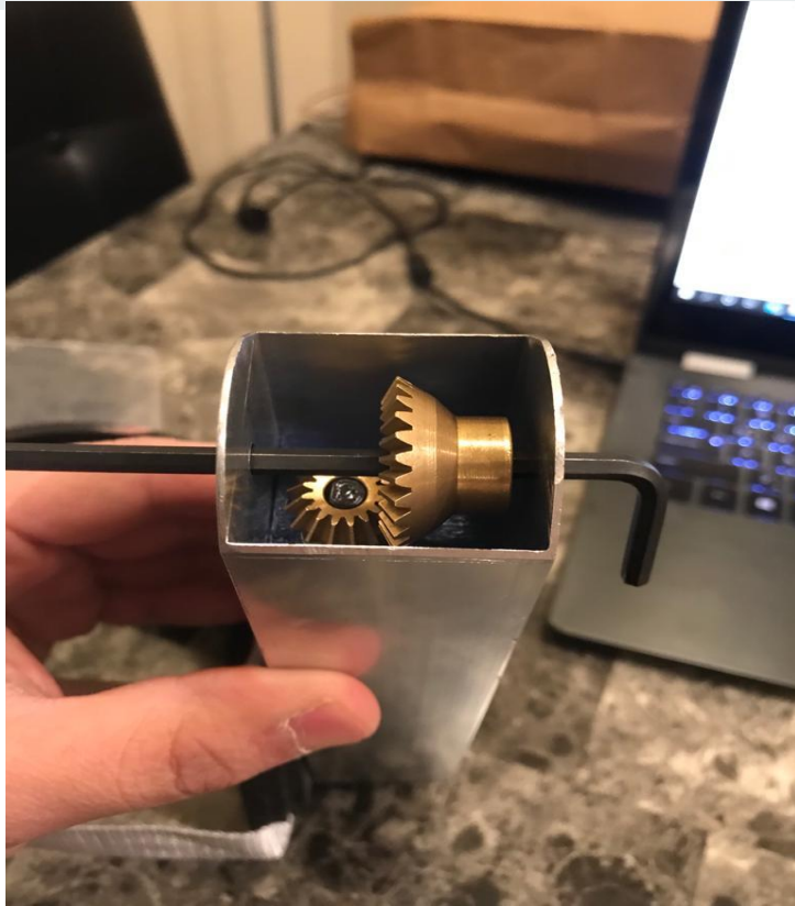
Figure 5: Gear connection inside the tube
